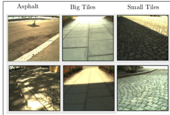
Figure 7-7: Sample images of Asphalt, Big Tiles, and Small Tiles under different lighting conditions with shadows to increase the classification complexity.
