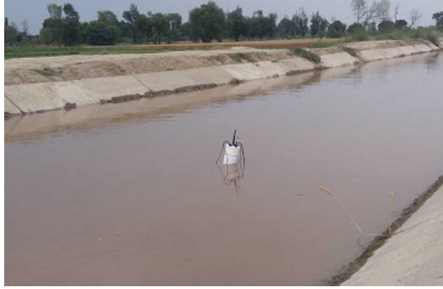
Figure 3-1: Lagrangian sensor equipped with GPS floating in a canal.
