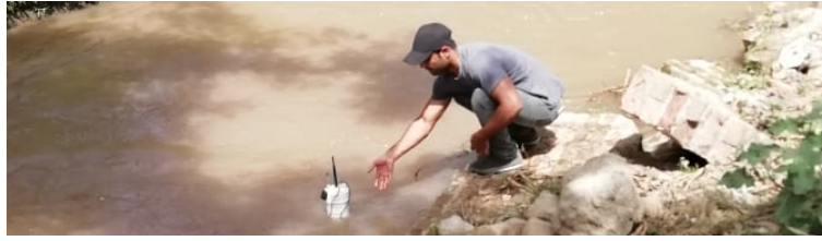
Figure 6-7: The release of mobile sensor into the water body at upstream end of experimental canal
