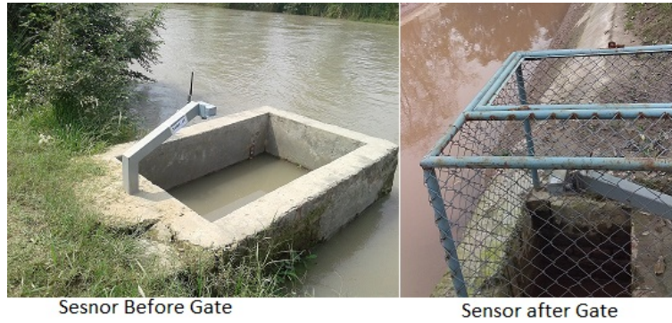
Figure 6-5: The static water level sonar sensors upstream and downstream end of the undershot gate at the start of canal.
