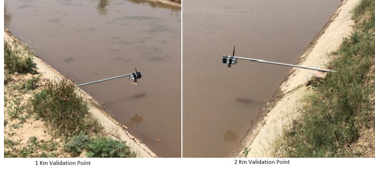
Figure 6-6: The static water level sonar sensors at 1 Km and 2 Km from sensor mounted at downstream of undershot gate.
